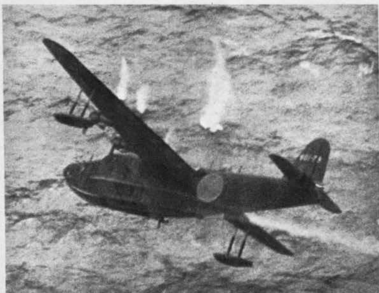
EMILY One of the Japs' most successful designs, Emily makes 245 m. p. h. at sea level, has 4,190-mile range. The nose is long and pointed. The single fin and rudder sit forward of tail gun.
